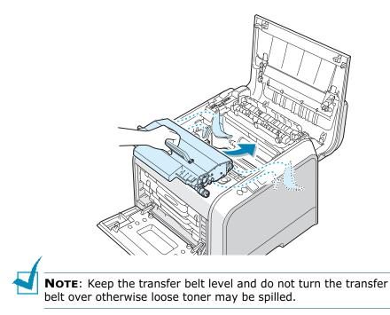
**11** Slide the new transfer belt down into the printer and press it firmly into place.
